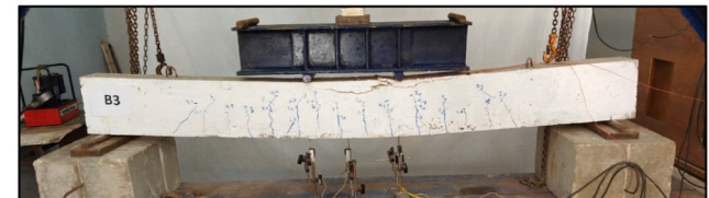
(c) Crack Patterns for the Tested Beam B3
