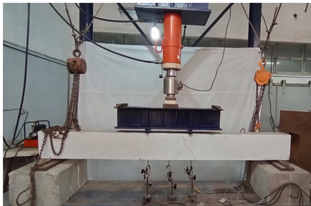
Fig. 5. Typical test setup for the beam specimens.
