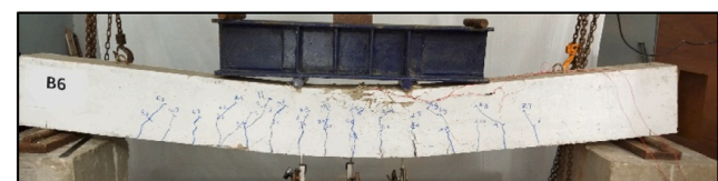
(f) Crack Patterns for the Tested Beam B6
